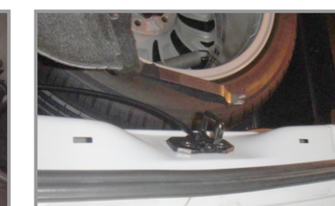
8.Dismantle original latch base and the install our latch base
