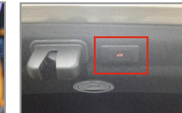
18.Install the rear button on the position as shown
