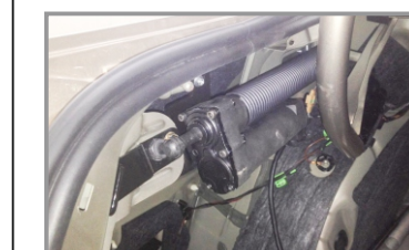
7.Install our electric poles
