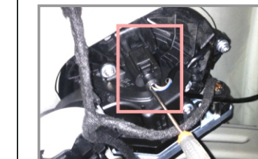
11.Take out the original button's cable and then joint with our button connecting cable
