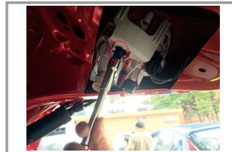
13. Unscrew the right tailgate light screw, then dismantle the right taillight.
