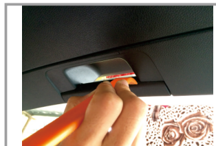
3. Dismantle the handle plaque, which is on the right of tailgate plaque.
