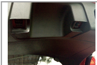
5. Dismantle the handle of tailgate plaque.
