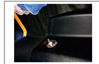
16. Remove the screw of lock latch plaque.
