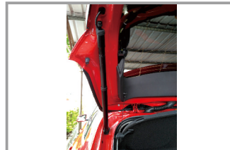
11. Install the electric pole (both the left and right one).
