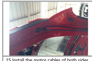
15. Install the motor cables of both sides poles and rubber plug of holes. (There is a hole on the left, it's no need to drill one, just install our rubber plug)
