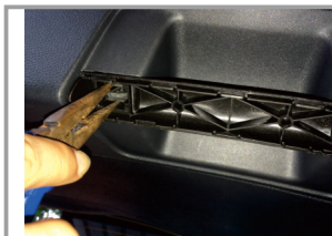
4. Clip the buckle with a sharp-nose plier, pull the handle.
