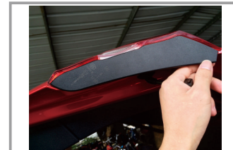
12. Pull down the right tailgate light plaque.
