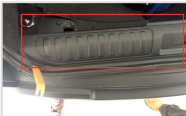
25. Dismantle the original plaque by tool
