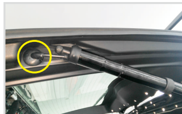
7. Dismantle original rubble plug (as shown) and install our poles
