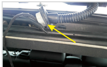
23. Wipe the professional waterproof glue after putting our wire harness through to the waterproof rubber hose
