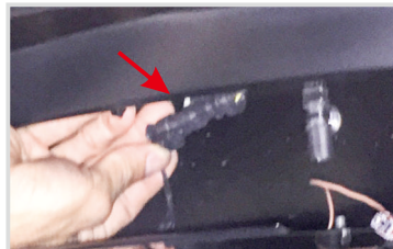
17. Take out the original plug and take off the car tail (as shown)
