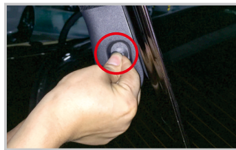
9. Take down the buckle of the hang plaque on the tail gate
