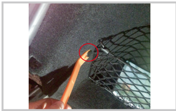
6. Take down the buckle of the plaque on the right side
