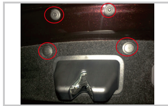
11. Dismantle all buckles on the tail gate
