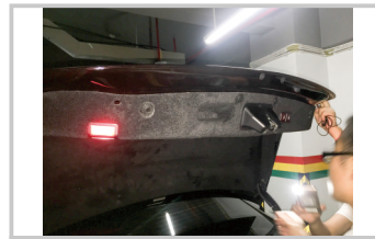
12. Take down the whole plaque of tail gate
