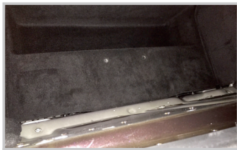
3. Take down the screws of trunk plaque, and take down the plaque
