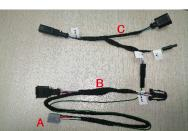
Lock control wire A. Control box port -1 B. Connect to the tailgate lock C. Connect to the tailgate handle button switch
