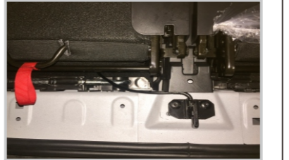
24. Install our company's puller lock latch stand (note: firstly take out the latch stand through the seats under) (use the original screws)
