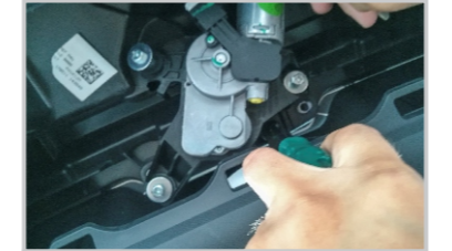
7. Dismantle the screws hiding behind the motor
