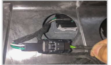
8. Converting joint to the press key of original tail door
