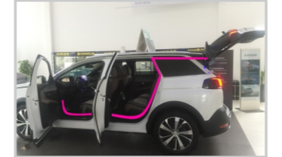
31. Arrange the cables to the tail door according to the method showed in the drawing
