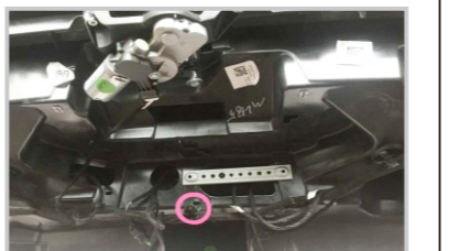
10. The installation position of control box bracket. Pry out the original buckles which are circled out in the drawing
