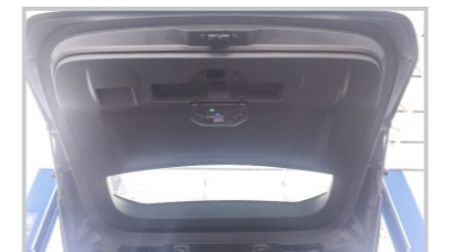
1. Dismantle the tail door decorative plate
