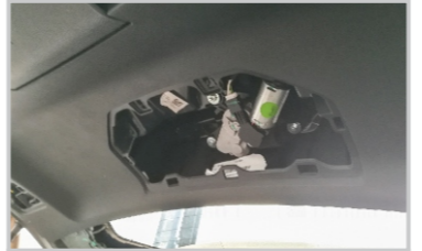
6. Dismantle the three screws for fixture of the windscreen wiper
