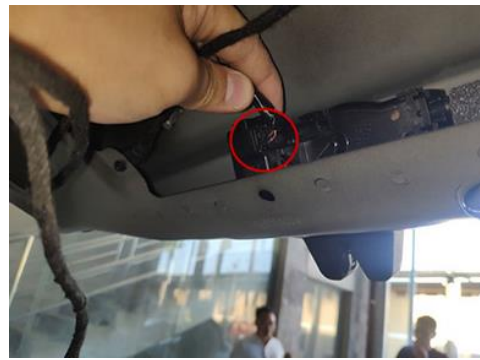
15. Pull out original lock signal joints And then contact with our wire harness.
