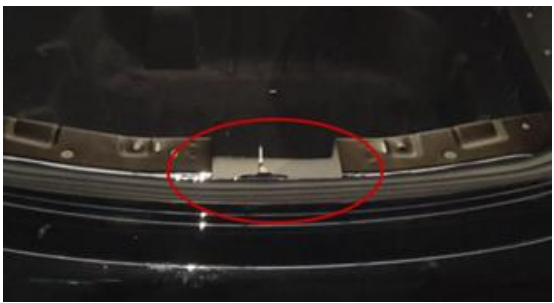
13. Assemble lower lock ring back, and screw stable on the car with M6 screws.
