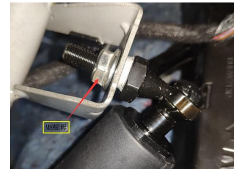
8. Install our ball head and M8 nut on the right side
