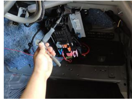
19. Move the fuse box for find the can line.
