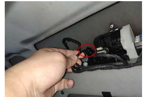
16. Pull out original rear switch joints And then contact with our wire harness
