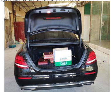
24. Installation restore, slowly manually close the tail gate, once the first time for system initialization.
