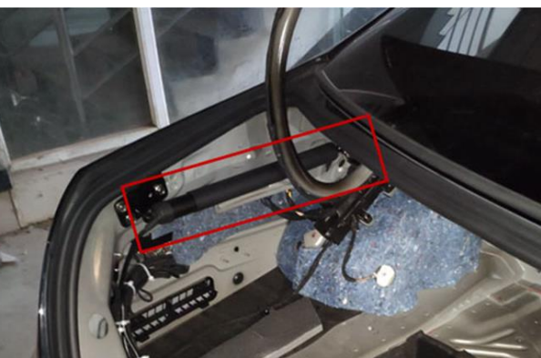
9.Install electric poles, same left and right.
