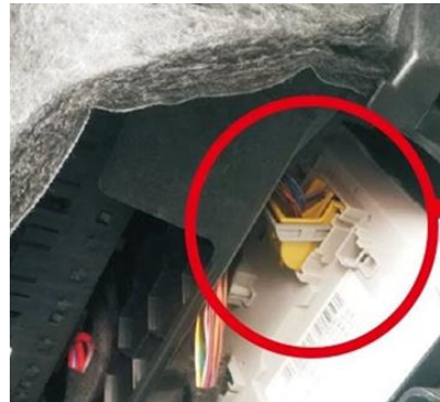
18. Find the Yellow plug behind the fuse box, Can line in this place.
