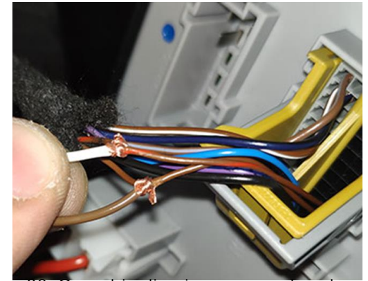
20. Our white line is connected to the original reddish brown line (CAN-H) Our brown line is connected to the original pure brown line (CAN-L)
