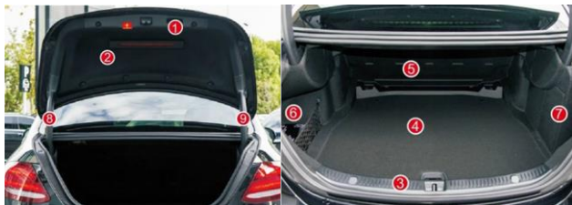
2. Remove trim panels in order .
