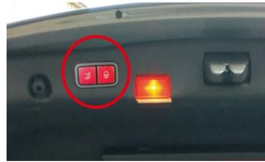
23. Install new specialize rear switch as shown.
