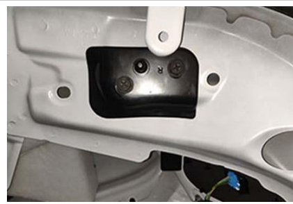
6. Install our body bracket ("L" on the left and "R" on the right)
