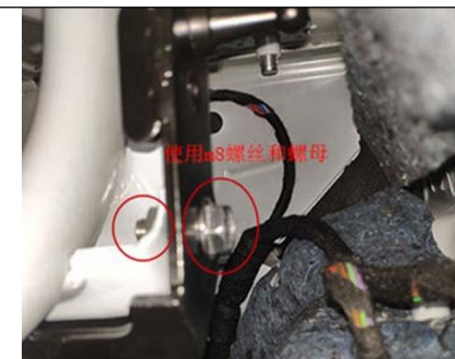
10. Use our M8 screws and nuts to lock in the original car suspension spring position (left and right are the same)
