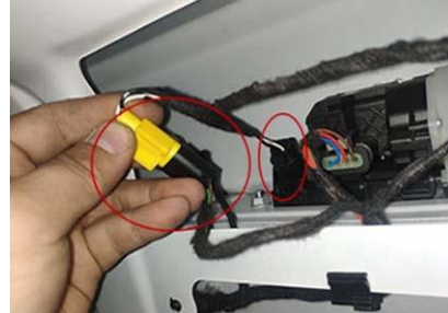
18. Unplug the original car lock plug and connect it to our wiring harness
