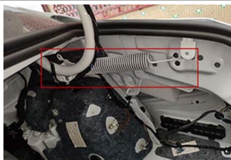
3. Remove the original car body spring (same for left and right)
