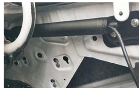
11. Install our electric brace ("L" on the left and "R" on the right)
