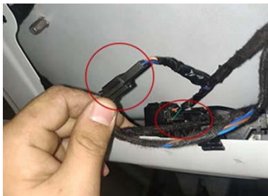
17. Unplug the original car lock plug and connect it to our wiring harness
