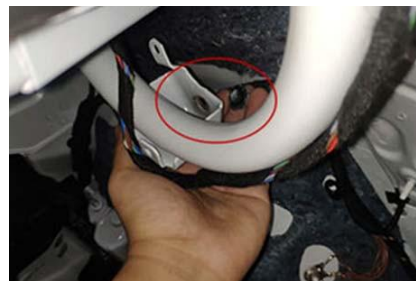
7. Remove the hanging spring plastic part (same for left and right)
