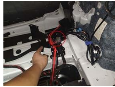
19. Find the wiring harness in the trunk
